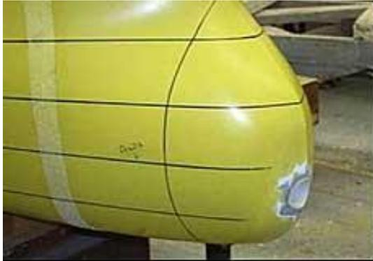
Two duct discharge locations tested in Marine Hydrodynamics Laboratory.
